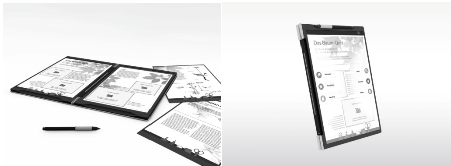
Fig. 6. "Mate" with displays taken out for more working space (left) or folded backwards as a mobile working station (right)
